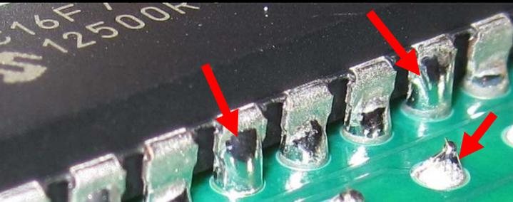
Solder (pronounced “sah-der”) is metal that can be melted to “weld” components to a PCB.
