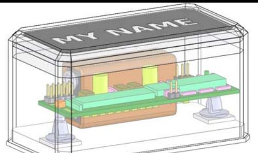
The electrical connections, called “traces” are laid out using a computer program before the PCB is made. The PCB has several layers, each with different traces. The layers are connected by holes drilled through all layers.
