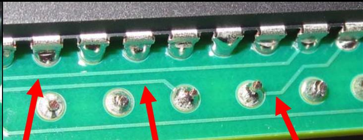
Thin copper traces make electrical connections. Green paint called “solder mask” protects them from damage.
